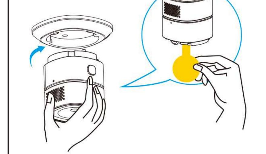
Anticlockwise rotating the bracket out from the installation base, then remove the battery insulating strip to make detector on power.
