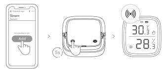
Tap "Add" on the main page of Zigbee Bridge on your eWeLink App, and long press the button on the device for 5s until the Zigbee signal icon (\*\*) flashes, now the device is entered the pairing mode and waiting to be added.
