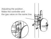
3.Put the valve controller on the gas valve and adjust. The drive arm should clamp the valve closely.
